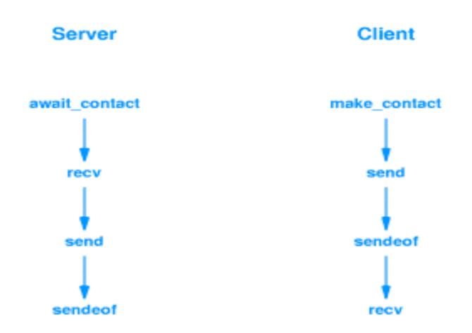
Figure 3.2 Illustration of the API calls used for a trivial interaction. The client sends one request and receives one reply.
