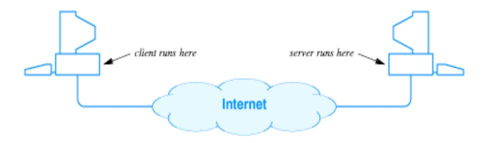
Figure 3.5 Illustration of the echo application, which can be used on any two computers connected to the Internet. The client program runs on one computer and the server program runs on another.
